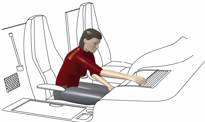
Figure 3, One of the final concepts where the guide area is separated from the entrance. A computer manikin is used for verification.
