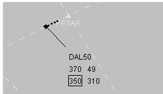
Figure 3: Data-link transmissions were indicated by a frame. The controller has issued flight level 350 and is waiting for a response.
