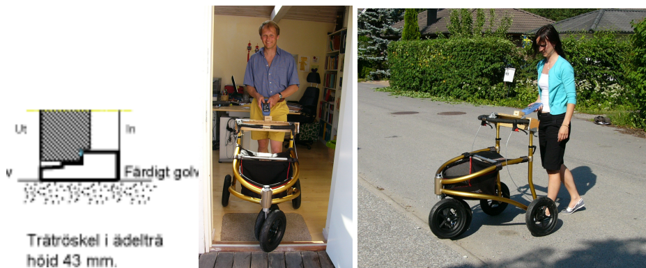
Figure 2: Cross-section of a standard threshold [left]. Traversing a threshold [center] and a curb [right] with the Walker prototype. The force is registered.
