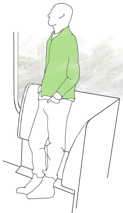
Figure 4: A Support for standing developed to give standing passengers of different length support at hip-height.
