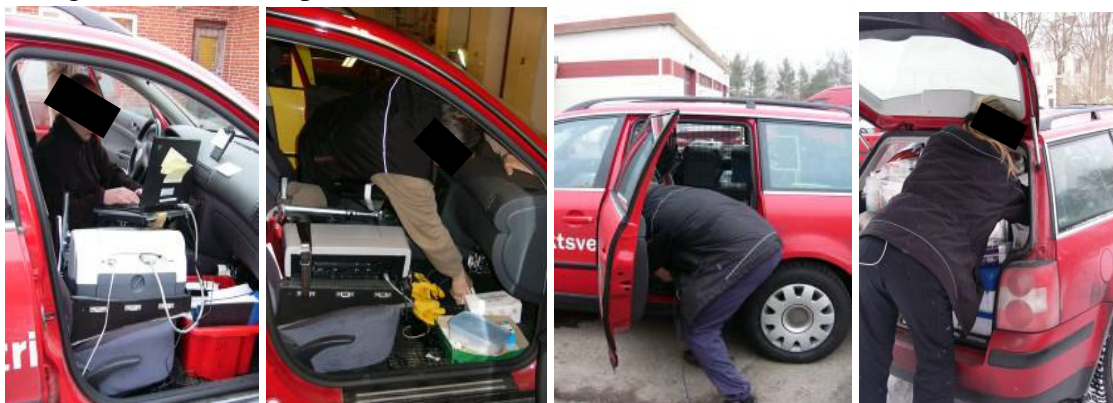
Figure 1: Examples of situations with increased injury risks a) equipment not secured during journey as well as the twisted working posture during computer work, b) installation of computer as well as c) manual material handling lead to unfavourable postures and d) unfavourable postures in combination with insufficient vision adds to the strain.
