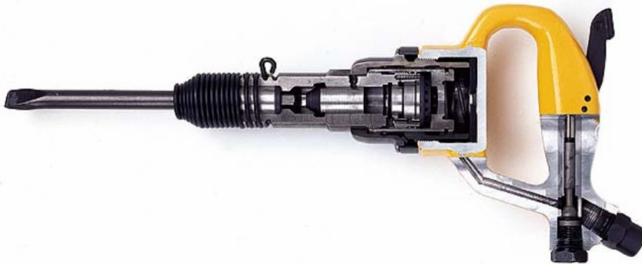
Fig 3 Chipping hammer isolated with a spring between the handle and the percussive mechanism
